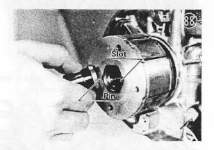
Align the projection on the engine sprocket lock washer with the hole in the sprocket, tighten down the mounting nut, and bend up one side of the lock washer.
