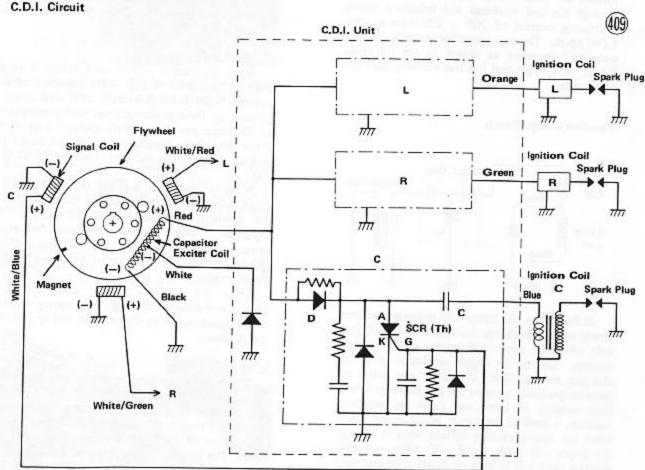
The chip of magnet is very small, but it has a strong magnetic flux. So when it cut through the coils instantaneously, the magnetic field in the coils changes so rapidly that a strong and sharp sine wave current is generated. This pulse current is sharp enough to trigger the thyrister in the C.D.I. unit without need of amplification. The three signal coils send signal current to ignite the spark plug in each cylinder at proper timing.
