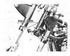
Tighten down the steering stem nut.
