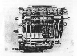
Tap the lower crankcase and shift shaft mounting lightly with a mallet, so that all the shafts, etc. remain in the upper crankcase when it is disassembled.
