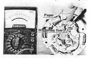
b. Check the contact points for wear or fouling. The points must be inspected periodically since they become worn after a long period of operation, and the slight sparking at each break gradually burns the surface.
