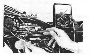
Secondary winding resistance between the spark plug cap and the ignition coil core is  $16 \text{ k}\Omega$ . If an inductance tester is available, inductance between the orange, blue or green and the core is 1.9 mh, and between the plug wire and the core it is 40 h.
