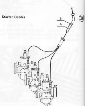
b. With the starter plungers in the fully closed position, adjust the outer sleeve of all starter cables for .04 — .08" (1-2 mm) play, in order to have all plungers start moving together. Adjustment is made with adjuster C while moving the cable sleeve up and down until only slight play is felt. Fix adjustment in place with lock nut D.
