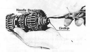
Remove the oil seals and bearings.
