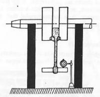
Under 0.0020 in. (0.050 mm)/4 in. (100 mm)
