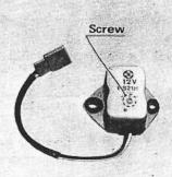
To avoid damage to the SVR, be sure the main switch is turned off before removing or replacing the unit.
