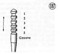
The first number indicates the length of dimension "a". The 5 in the example stands for 50 mm and over, but under 60 mm. A four would mean from 40 up to 50 mm and so on.
