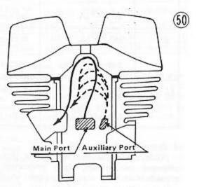
In the S and KH Series, the four-port scavenge method is employed to increase output power.
