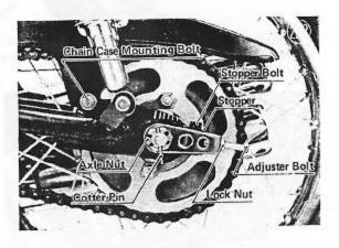
Disconnect the brake cable from the cam lever. Fully loosen both chain adjusters. Remove their bolts and take out the chain adjuster stoppers. Push the wheel forward to slip the chain off the sprocket, and then pull off the wheel.
