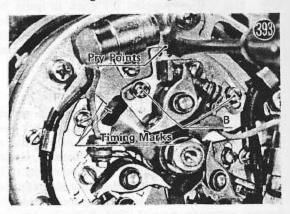
This adjustment must be done for each of the three sets of points to completely set ignition timing. When the L marks are aligned, for example, the L contact breaker plate mounting screws should be loosened and plate L pried, etc.
