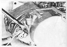
Remove the oil pump banjo bolts and take off the three outlet oil pipes.
