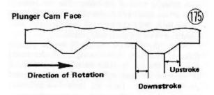
When the lowest part of the control cam is facing the plunger as shown in Fig. 174D, the plunger tip never touches the control cam and the cam on the plunger face can ride at point  $\otimes$  from its highest to lowest point — the distance between the arrows. Accordingly, maximum plunger stroke occurs at maximum throttle opening.
