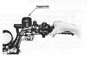
The correct fluid will come in a can labeled D.O.T.3. Do not use fluid that does not have one of these markings.
