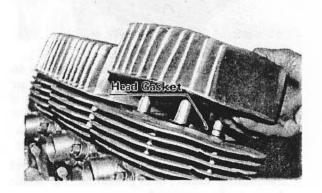
Pull the cylinder off the studs.
