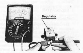
(ii) Connect the bulb between the regulator yellow/green lead and the voltage source + terminal. Connect the regulator black lead to the voltage source — terminal. Set the multi-tester to the 30 VDC range, connect the meter — lead to the regulator black lead, and connect the meter + lead to the regulator yellow/green lead.
