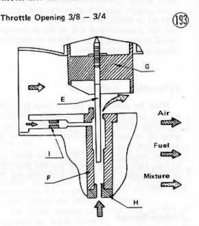
Among possible causes of faulty functioning would be obstruction or loose mounting of the main jet or needle jet, clogging of the air jet or needle jet, and jet needle wear.
