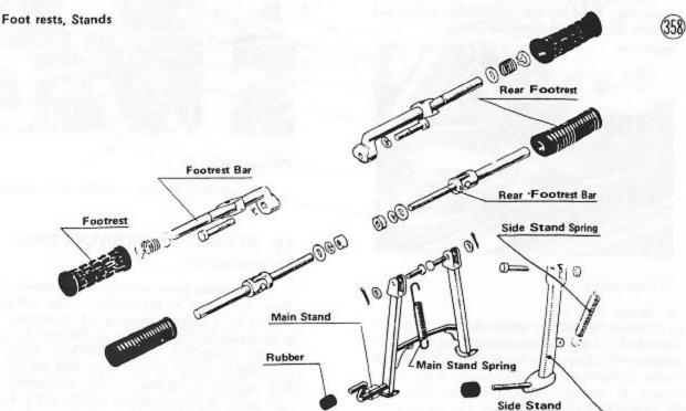
b. Take the spring off the center stand, pull out the cotter and joint pins, and remove the stand.
