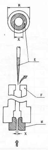
As in paragraph "c", any trouble might be due to clogging or loose mounting of the main jet, or blocking of the air jet, air passages, or needle jet. If after ascertaining the absence of clogging or loose mounting, the carburetor still does not function properly, the main jet must be adjusted by replacement. It should be kept in mind that the main jet is used during lower speeds as well as at open throttle, so there are limits to the amount of adjustment that can be made.
