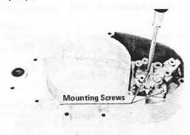
Take out the tachometer gear mounting bracket screws and remove the bracket, oil pump gear, shaft, and thrust washer.
