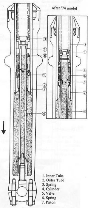
limit, replace it. If the length of the replacement spring and that of the remaining old spring vary greatly, replace both old springs to keep the shock absorbers balanced and thereby maintain motorcycle stability.
