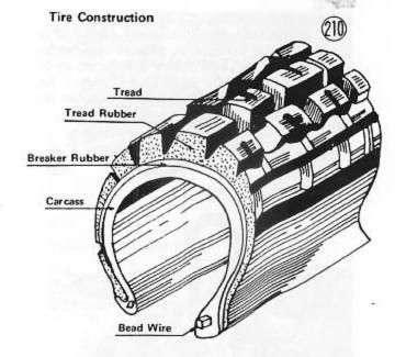
A rib pattern resists side slippage, and is usually used on the front tire. A tire with a block pattern tread has greater friction with the road surface and is therefore employed chiefly on the rear to improve braking and acceleration efficiency.
