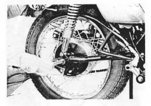
The coupling is separate from the wheel and drum, so when removing the wheel it is not necessary to remove the coupling.
