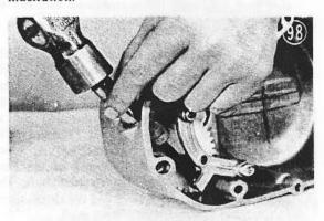
Transmission oil drain plug installation torque 37 – 52 ft-lbs (5.1 – 7.2 kg-M).
