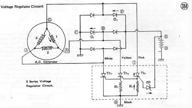
During each cycle of alternating current where the voltage exceeds 15 volts, the zener diode starts conducting at 15 volts, and stops conducting when the voltage drops below 14.5 volts. The thyristors start conducting when they are gated, and stop conducting each time the voltage reaches the negative half of the cycle.
