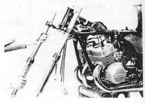
Take out the spring and pour out the oil. The oil can also be removed with the fork still attached to the frame, by removing the screw at the bottom of the fork and draining the oil.
