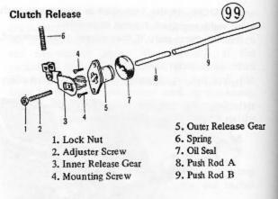
The clutch release mechanism on KH400 is shown in Fig. 100. The clutch release outer worm gear and the inner worm gear are made of steel. Balls are installed between the outer and inner worm gears to reduce the friction between them. Assembled into the center of the release inner gear is the clutch adjusting screw, which pushes on the push rod and spring plate pusher the drive shaft to release the clutch.
