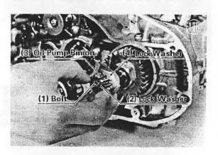
Straighten out the lock washer.
