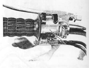
Remove the clutch and brake lever assembly.
