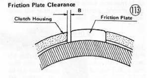
Table 14 Clutch Housing/Plate Clearance
