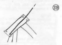
To remove the inner race from the steering stem, set a cold chisel to the point where the race and stem meet and hammer on the chisel lightly, moving it to different points so as to remove the race evenly. Be careful not to hammer too heavily as the stem will become misshapen.
