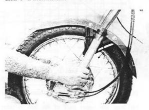
If the preceding inspection revealed play in the steering stem, the lock nut is not tightened sufficiently; if the steering was stiff, the lock nut is too tight and must be loosened.
