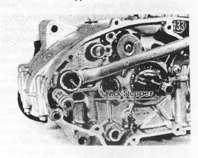
Turn the crankcase assembly upside down and remove the mounting nuts.
