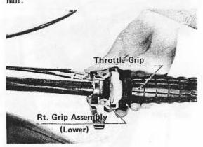
Remove the throttle and starter cable wires.
