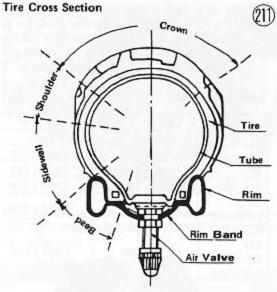
The tire size marking shows tire dimensions in inches. For example a 3.00–18 tire has an overall width of 3.00 inches, and fits on an 18 inch rim, i.e. its inside diameter is 18 inches. An "S" after the width number indicates a tire for high speed use.
