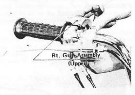
Pull the throttle grip off together with the bottom half.
