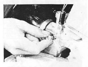
(3) With all the throttle valves fully closed, adjust the outer sleeve of each throttle cable for zero play. Accomplish this by turning throttle cable adjuster C right or left, while moving the cable sleeve up and down until no play is felt. Don't fail to tighten lock nut D after adjustment is made.
