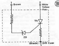
(3) Connect a 12 volt battery between ③ and ① with the negative lead to ③ and positive to ①, as shown in Fig. 387. Use an ohmmeter (tester) to see that current will not flow from ③ (-) to ①(+). If current flows, the zener diode is defective.
