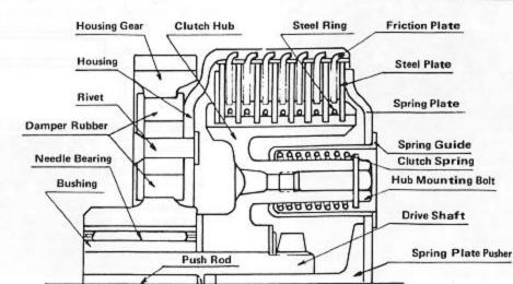
Take off the lock washer and flat washer. Remove the clutch hub, thrust washer and clutch housing from the drive shaft in that order.
