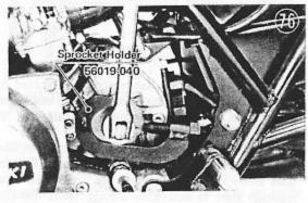
c. AC Generator Stop the crankshaft from turning and follow these steps:
