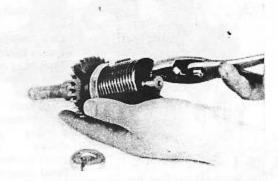
Remove the snap ring and take the kick gear and holder off the kick shaft guide.
